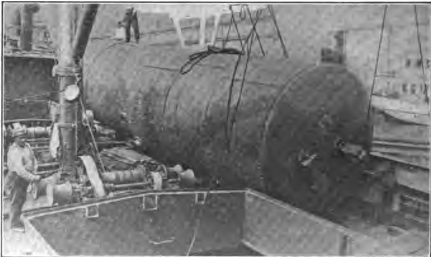
FIG. 145.—Crystallizers (for sugar factory) 9 ft. diam. \times 22 ft. long on deck of small steamer.
